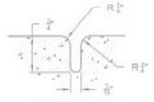
WEAKENED PLANE JOINT DETAIL
