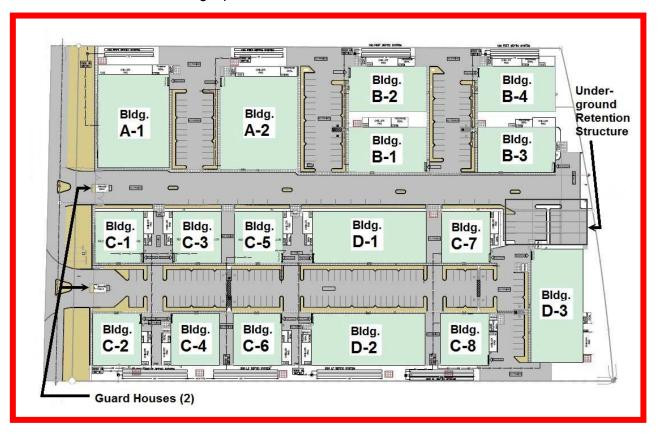
2. Paved vehicular circulation is proposed throughout with two main drive aisles accessing Little Morongo Road and multiple dead-end drive lanes projecting from the main aisles. Among the northerly buildings (A-1, A-2, B-1 thru B-4) the main drive aisle runs along the south edge of the six buildings, with three dead-ends projecting to the north and one loop aisle in the rear (easterly end). Among the southerly
